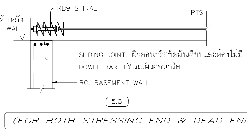
5. TYP. REINF. AT JOINT BETWEEN SLAB & RC. BASEMENT WALL
